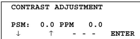
This enables you to adjust the brightness by pressing the [F1](↓) or [F2](↑) key.
