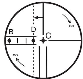
3) Shift the vertical cross-hair line and coincide it with Point D, by revolving the left and right capstan adjustment screws with the adjusting pin. Upon completing the adjustment, repeat the checking operation once more. If Points B and C coincide, further adjustment is not required. Otherwise, repeat the adjustment.
